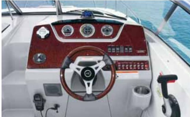
SmartCraft® instrumentation with built-in engine diagnostics come standard. A VHF radio is optional.
