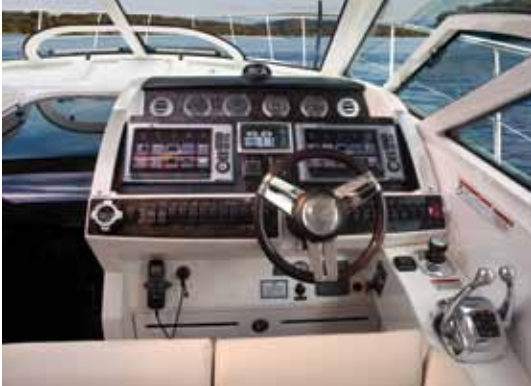
The fully equipped control station features SmartCraft™ diagnostics and VesselView display, plus optional Raymarine® E125 widescreen radar/GPS/chartplotter and dual displays.
